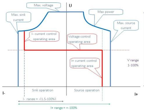
EPS/TSDCR Ausgang/Output characteristic
